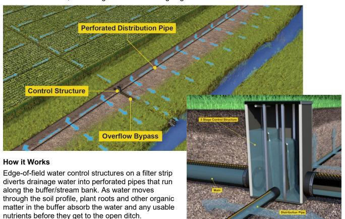
In times of high flow, the water can bypass the buffer by flowing over the stoplogs to a traditional tile outlet. This bypass ensures the water table isn't backed up too far into the field, so the tile system functions as a typical controlled drainage system.
